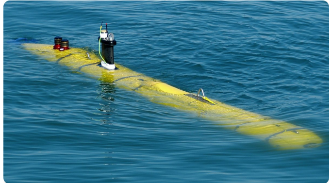
Fig. 1. Bluefin 21” AUV with dual Sonardyne AvTrak6 HP modems for redundant acoustic communication.
